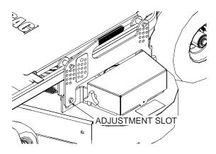
Figure 6-2. Cutter Deck Adjustment Slots
